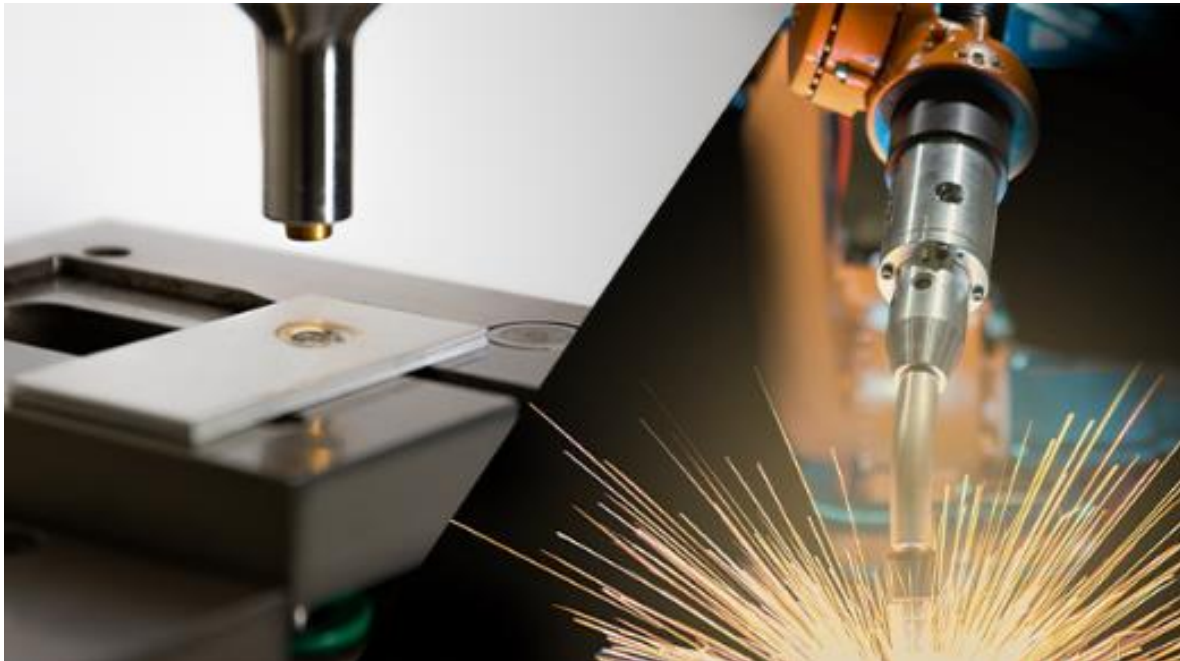
Image 1: An examination conducted by the laboratory for materials engineering and joining technology of the University of Paderborn showed that there is significantly less energy consumption during clinching compared to resistance spot welding.
